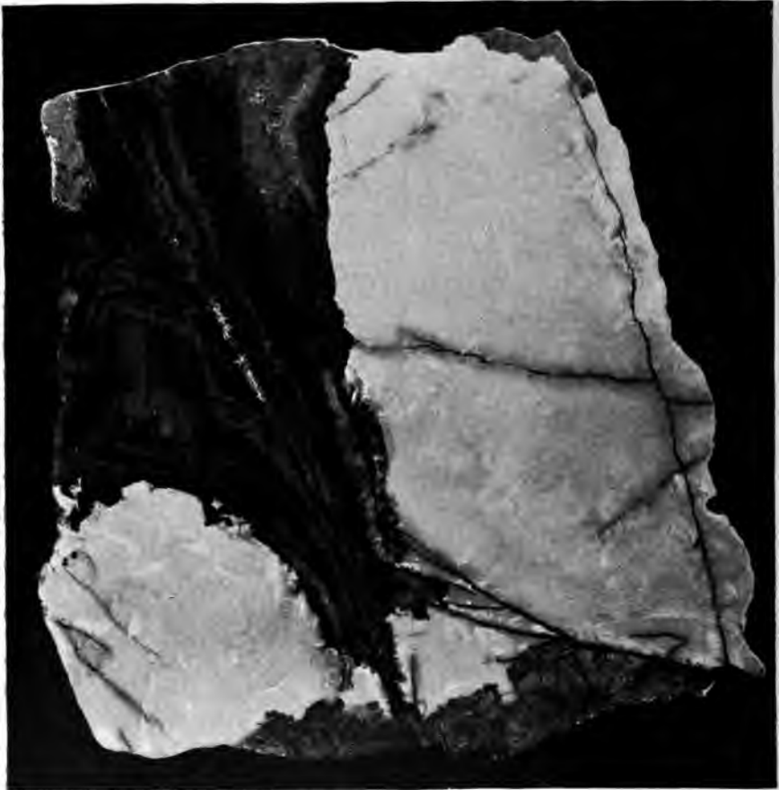
SLAB FROM SAME BLOCK AS SHOWN ON PLATE 5, BUT SHOWING A MORE ADVANCED STAGE OF OXIDATION.
